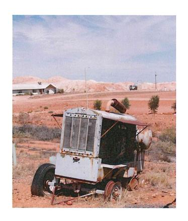
Leroi compressor built during the 1950's in Milwaukee Wisconsin USA. Featuring 4 cylinder petrol engine with updraft carburation powering a 3 cylinder radial compressor. The machine also features a radiator constructed by the Young Radiator Company of Racine Wisconsin USA.
