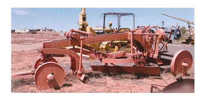
These Graders were built in Sydney (Australia) by Armstrong Holland during the 1930's, 1940's and 1950's. They were originally towed by a small dozer or larger tractor and widely used throughout Australia in road construction. Armstrong Holland had an associated business called Champion Construction Machinery, also operating out of Sydney (Australia)
